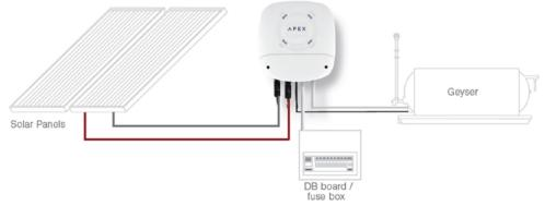
Figure 1. SGS PV hot water controller system overview
