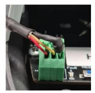
Figure 7. Temperature Sensor's Connections To The SGS PCB
