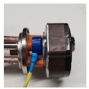
Figure 6. Temperature Sensor Installation
