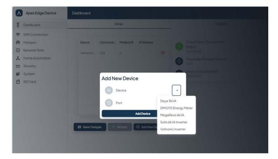
From the Device list, choose your supported device. The Port will automatically be assigned, according to the available driver.
