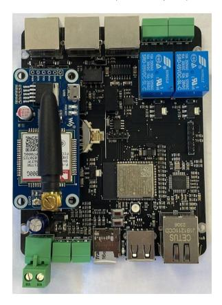
Remove the antenna from the module by unscrewing the nut.
