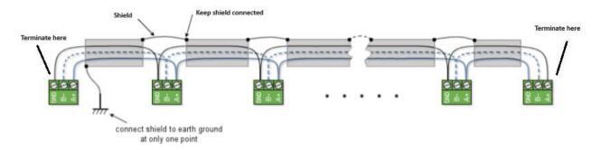
Always terminate both ends of the bus and never terminate elsewhere. Incorrect bus wiring will result in the device failing to communicate or communicating erratically.
